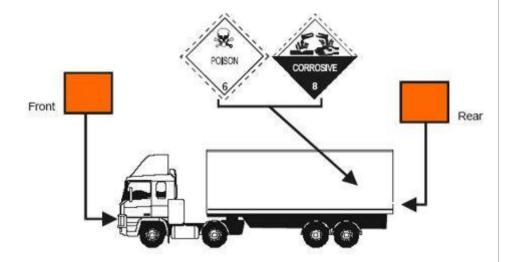
The image above shows signage for a vehicle carrying dangerous goods in packages in a demountable freight container. In addition to the orange panels to the front and the rear of the vehicle all sides will have the standard warning signage according to the load carried.
