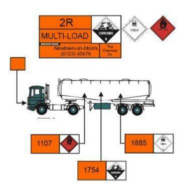
The image above shows the signage for a multi load tanker. The main placard will state multi load but the hazard symbols will show the hazards of the load. Each individual compartment of the tanker will have its own signage giving the UN number for the substance and the hazard symbol denoting its specific hazard.
