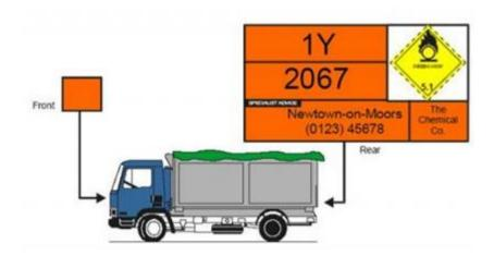
The image above shows the signage for a bulk single load in excess of 3 cubic meters. The detailed signage will be on the sides and rear of the vehicle
